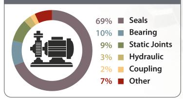
According to *Pump and Systems Magazine* and the FSA Mechanical Seal Technical Committee.
